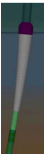
Figure 12.17 Flexible Riser System - Bend Stiffener
